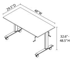
**NOTE:** Desk includes one crank. Second crank shown for visualization of crank mounting points.
