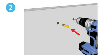
Using the markings created with the drilling template, drill 4 holes with a 3/16" drill bit. After drilling, insert a plastic wall anchor into each of the holes.
