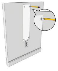
Using the drilling template, mark the location of the charging hub. **TIP**: Place the hub directly above an available wall outlet, if possible.
