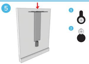
Align the keyholes on the top rear of the column to the mounting screws on the wall. Slide the unit down so the screws sit snugly inside the keyholes, as shown. Once properly positioned, the mount holes at the bottom of the column should line up with the remaining 2 wall anchors. Once aligned, secure the charging station using the remaining mounting screws.
