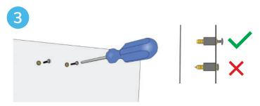
Drive mounting screws into the top two wall anchors. Do not drive them until they are flush against the wall. Leave a gap of approximately 1/8".
