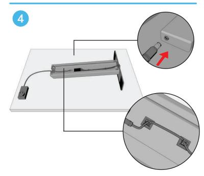
Set the charging station face down on a flat surface. Connect the power supply then secure the cord to the inside of the column using the supplied zip ties and pads.
